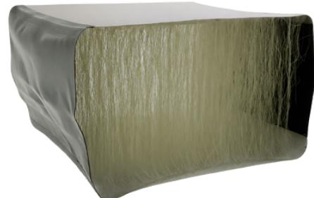
The power of drop stitch performance lies in a precision-built internal core: two fabric layers held apart by tens of thousands of high-tensile fibers. When sealed and pressurized, those fibers lock in place, forming an exceptionally stiff, perfectly flat surface that traditional inflatables simply can't match.
